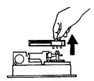
4) Holding new cartridge over spindles with black band up and exposed portion of ribbon on side nearest print wheels, place cartridge on spindle and engage cartridge.
