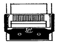
3) Lift out cartridge by moving the lever to the center, then move and lift out the cartridge.
